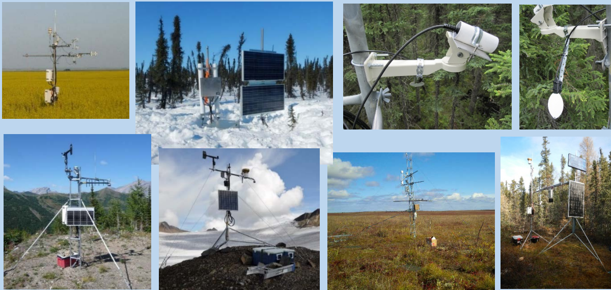
Figure 3: Photographs of new or enhanced hydro-meteorological observation stations at some of the WECC observatories. Top row from left: meteorological station at Brightwater Creek, cosmic ray soil moisture and snowpack monitoring equipment at Trail Valley Creek, infrared thermometer and leaf wetness sensors at BERMS. Bottom row from left: meteorological stations at Fortress Mountain ridgetop (part of the Canadian Rockies Hydrological Observatory), Brintnell-Bologna Icefield, Trail Valley Creek tundra site, and Baker Creek (including a Campbell Scientific GMON3 snow water equivalent sensor). There are dozens of other new or enhanced stations at the various WECC observatories.
