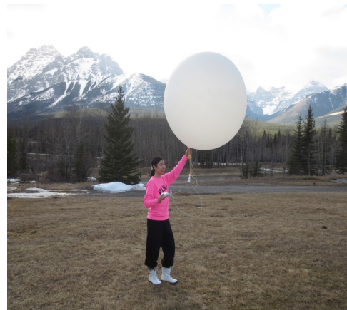
Ida gets ready to release a radiosonde balloon to retrieve information on the vertical profile of the atmosphere.
