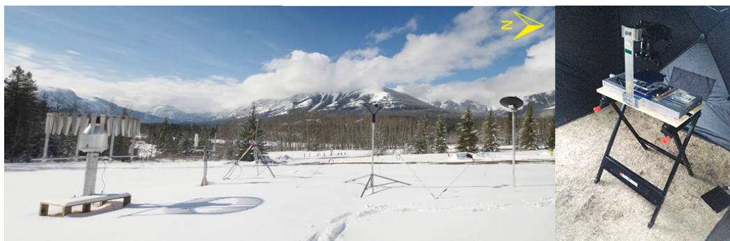
Instrumentation used in Ida's research, including (L-R) geonor with alter shield, sounding system, optical disdrometer, Micro Rain Radar, and microphotography.
